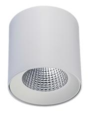
The Stark Mini LED is a 117mm diameter surface mounted downlight which uses a CREE LED engine. The heatsink is constructed from die-cast aluminium complete with aluminium rolled-formed body and reflector. The base plate uses three fixing points with a twist and lock action to secure the luminaire on the ceiling. The bezel has a deep recess detail creating a glare friendly cut-off which is also an aesthetically pleasing architectural detail.
