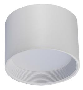
The Stark is a 195mm diameter surface mounted downlight which uses a CREE LED engine. The heatsink is constructed from die-cast aluminium complete with aluminium rolled-formed body and reflector. The base plate uses three fixing points with a twist and lock action to secure the luminaire on the ceiling. The bezel has a deep recess detail creating a glare friendly cut-off which is also an aesthetically pleasing architectural detail.
