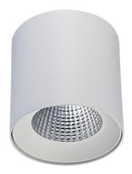
The Stark LED is a 200mm diameter surface mounted downlight which uses a CREE LED engine. The heatsink is constructed from die-cast aluminium complete with aluminium rolled-formed body and reflector. The base plate uses three fixing points with a twist and lock action to secure the luminaire on the ceiling. The bezel has a deep recess detail creating a glare friendly cut-off which is also an aesthetically pleasing architectural detail.
