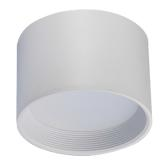
The Stark Mini LED is a 130mm diameter surface mounted downlight which uses a CREE LED engine. The heatsink is constructed from die-cast aluminium complete with aluminium rolled-formed body and reflector. The base plate uses three fixing points with a twist and lock action to secure the luminaire on the ceiling. The bezel has a deep recess detail creating a glare friendly cut-off which is also an aesthetically pleasing architectural detail.
